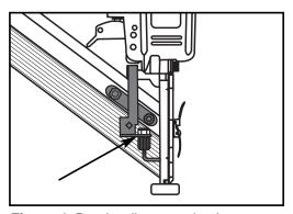
Figure 4. Depth adjustment knob.
